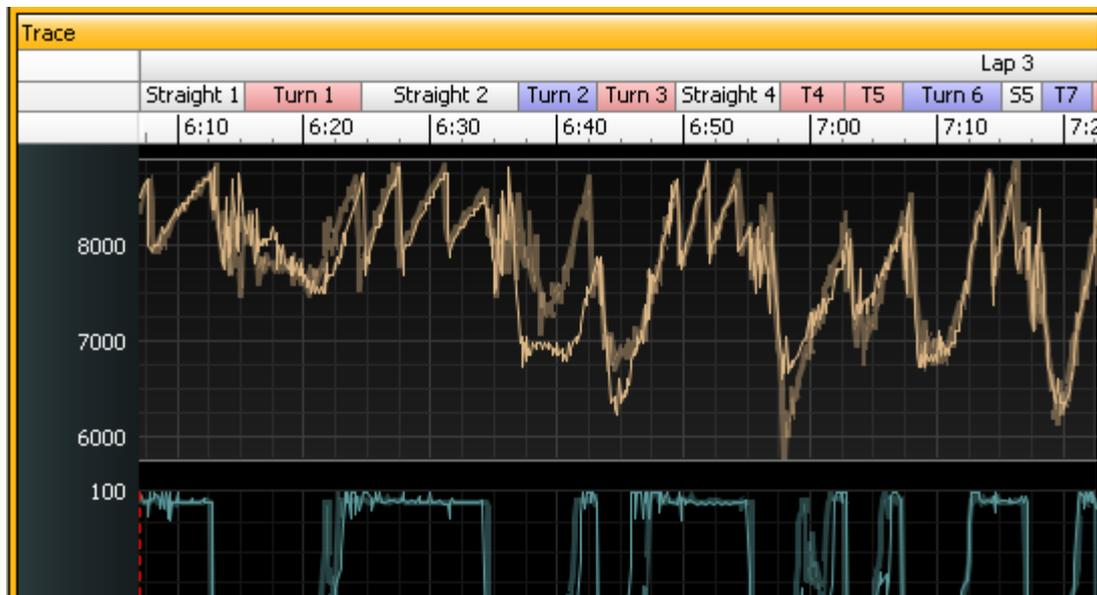
Setting up the trace can be done in two ways. Firstly by dragging channels from the Channel List. Click and hold, on a channel in the Channel List then move the mouse over the trace:
